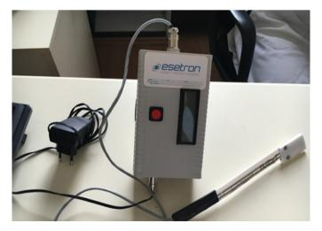
Figure 2: Jaw bite force measurement device
